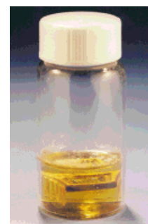
Figure 3. Encapsulated test microchip from a 80:20 copolymer mixture of 2 and 1 .
